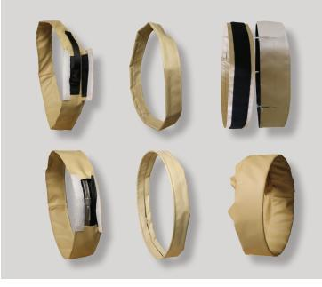
In order to combat everyday wear and tear associated with the most common failure points, wear strips, also known as scuff strips, can be added to the ducting to protect the areas where the internal wire may cause additional duct wall damage. One inch wear strips are attached to the outside of the ducts during the manufacturing process.
