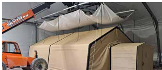
Snow load validation accordance with TOP 10-2-175
