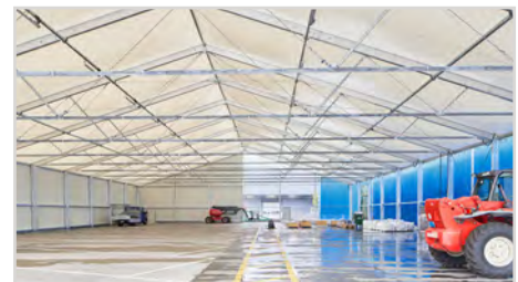
Pre-Engineered aluminum alloy frame support system
