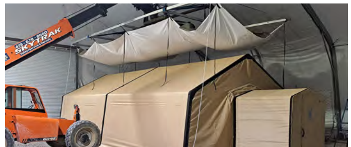
Snow load validation accordance with TOP 10-2-175
