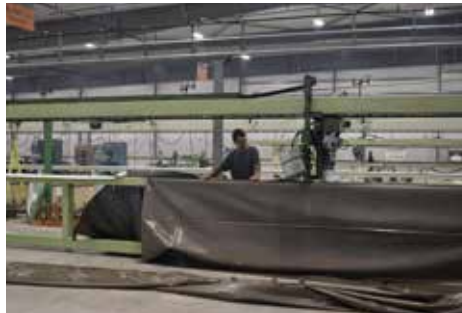
Hot air fabric welding equipment with alignment lasers & vacuum beds for holding fabric in place.
