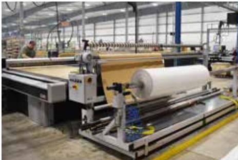
CNC fabric cutting and marking machines use CAD model interfacing to cut fabric with print integration and lot control marking.
