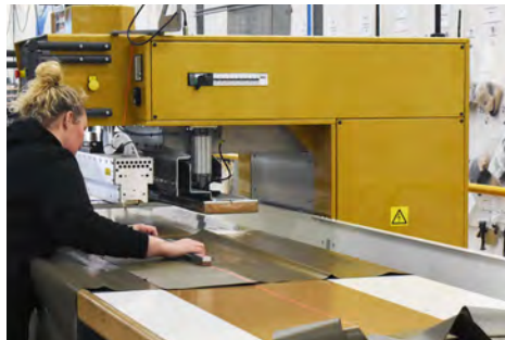
Fabric layout, inspection, and welding using HF/RF welding equipment.
