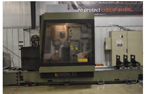
CNC machining center uses CAD model interfacing to fabricate metal frame components.
