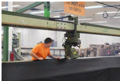
Hot air fabric welding equipment with alignment lasers & vacuum beds for holding fabric in place.
