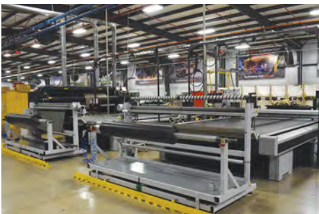
CNC fabric cutting & marking machines use CAD model interfacing to cut fabric with print integration and lot control marking.
